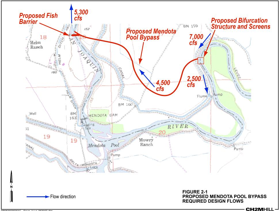
Additional Considerations. Conveyance of flows in the San Joaquin River above 2,500 cfs downstream of the Chowchilla Bifurcation Structure will require changes to the flood bypass operating criteria.
