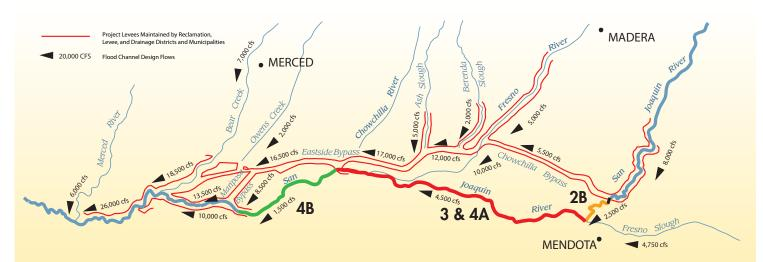
Restoration plans propose that all channels on the San Joaquin River have a minimum flow capacity of 4,500 cfs, which would require an increase in flow capacity of Reach 2B and 4B and evaluation of flow capacity in Reach 3 and 4A.
