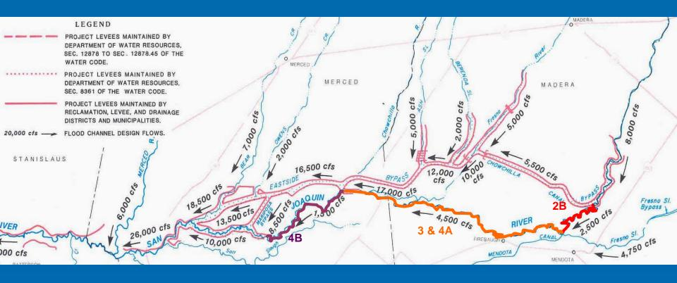
Restoration plans propose that all channels on the San Joaquin have a capacity of 4,500 cfs. This means increased flow capacity in Reaches 2B and 4B and evaluation of the design flow capacities in Reach 3 and 4A.
